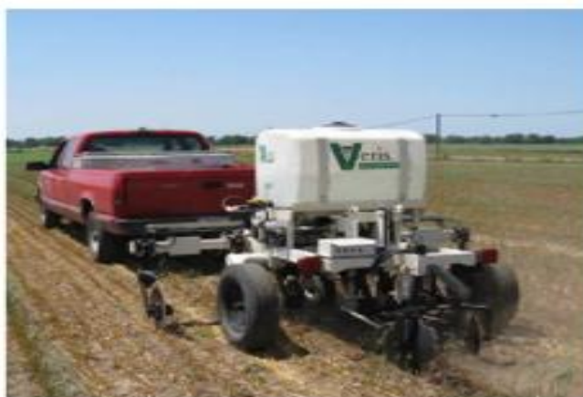
Electrochemical sensor for soil pH mapping
