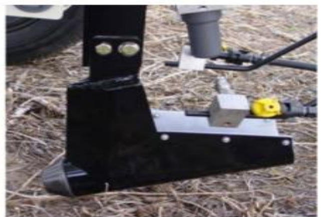
Electrochemical sensor for soil pH mapping
